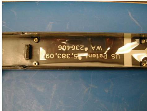
4. Replacement is reverse of removal. When installing the new MCU board, make sure it is properly laid over the pem studs.
