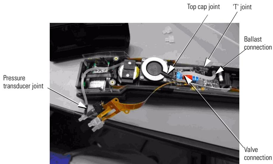
4. Observe leak rate again. If leak rate remains constant or increases the leak is in the pressure transducer area. Repair leak and retest. If leak rate stops, remove hemostat and proceed to step 5.
