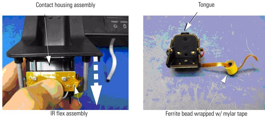
3. To remove the IR flex assembly, unsolder the four wires from the IR board. Observe color for each location.
