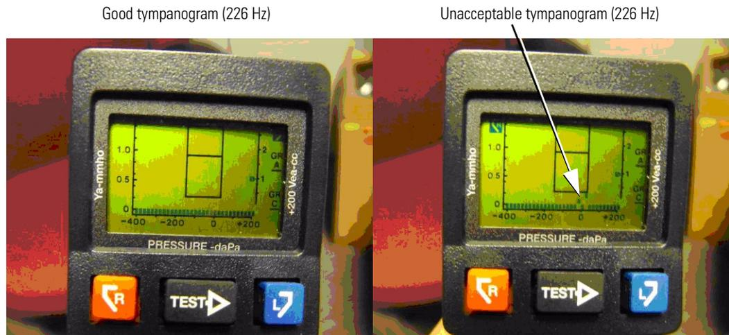
Test 3 - Compliance check for 226 Hz function only
