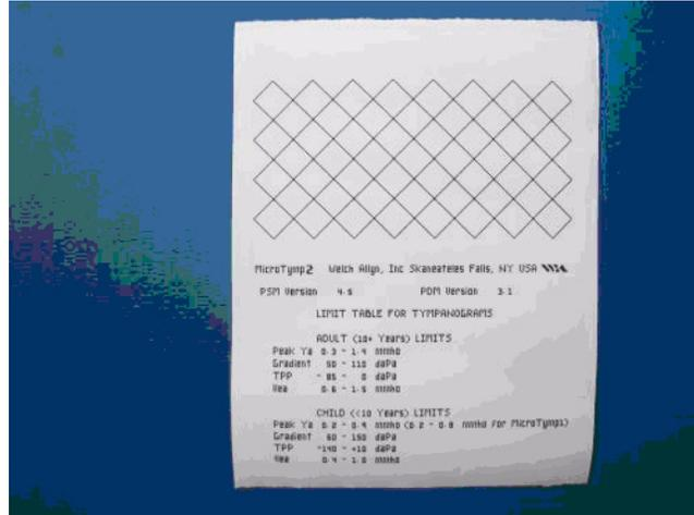
2. Make sure there are no gaps in the grid printout and that all lines of data are full with no lines missing through the lettering.
