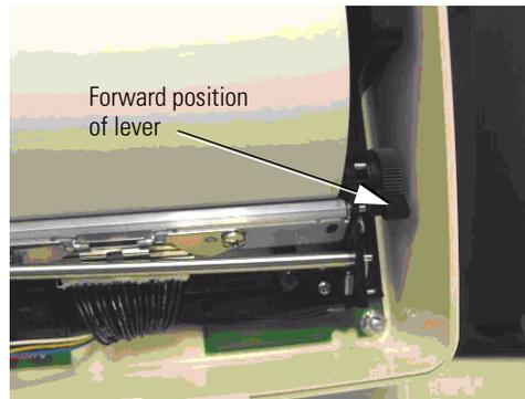
8. Push lever all the way back. Power light should stop blinking and stay on. This is normal operating mode for the Printer/Charger.
