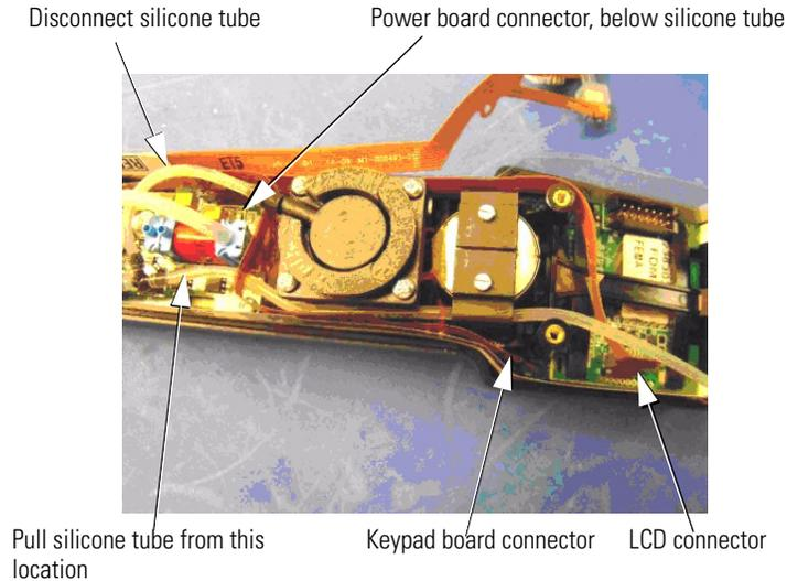
Once the pump motor assembly has been removed, another one can be installed or the assembly can be further dismantled.
