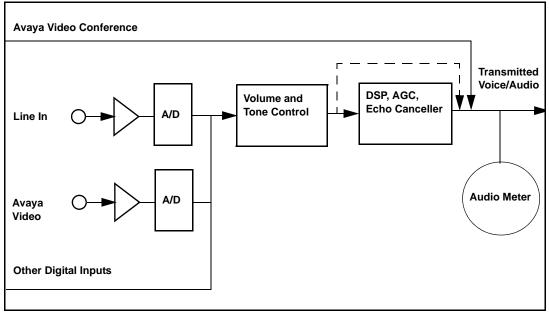
The dotted line illustrates the audio path when *Microphone In (No AEC)* or *Line In (No AEC)* is selected as the active microphone. This mode is useful for setting up system gains but should never be used during calls unless the installation includes audio inputs with external AEC. Echo may occur if no AEC is employed.
